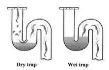
Anyone who is concerned about potential sewer gas entry into their home can take precautions to fill their plumbing traps with water periodically to prevent them from drying out. Every drain line should have a u-trap which holds water to prevent gas and odor from the sewer backing up into your building. If some drains are not used regularly, they may dry out and allow sewer gas and odor to enter your home.
