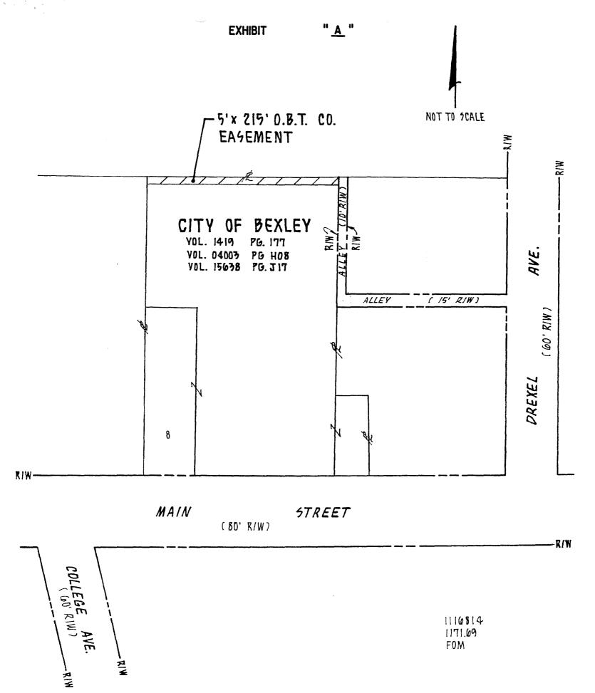
This Exhibit is Drawn For The Limited Use Of The Ohio Bell Telephone Company To Identify The Easement Location And Is Not Intended To Represent An Accurate Survey Of The Property.
