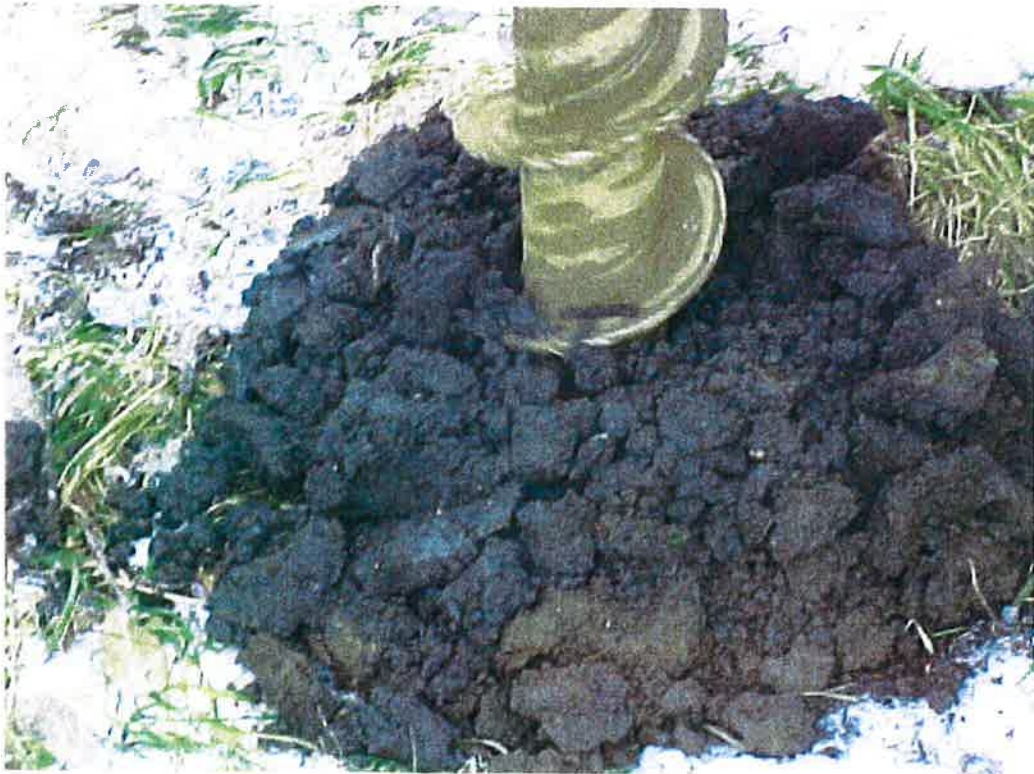
Photograph 6: View of soil clippings from geo-technical boring containing glass and metal fragments.
