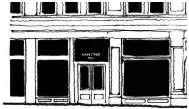
Figure 17.2 • Storefront Detail - storefront should relate directly and clearly to the public street with a minimum of 60% of the storefront consisting of transparent window and door glass
