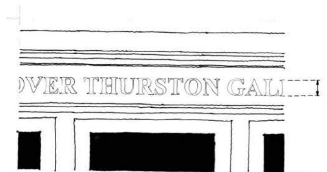
Figure 25.6 • Wall Sign Lettering - lettering should be between 18 inches and 26 inches in height and occupy no more than 65% of the sign
