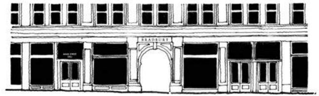
Figure 17.1 • Multiple Storefront Facade - storefront facade shall be divided into narrow bays with entryways recessed into the facade line
