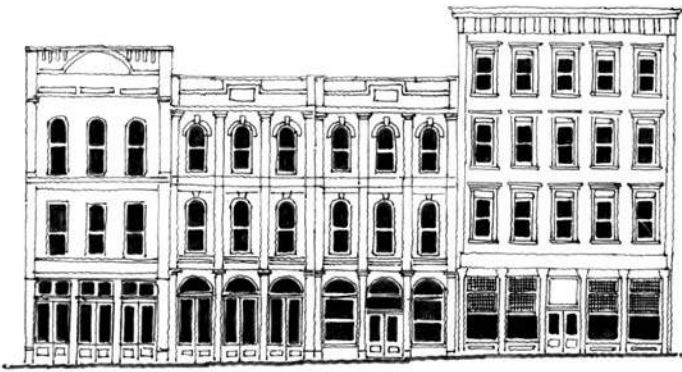
Figure 13.1 • Building Massing - buildings on Main Street should compliment the massing of traditional blocks on commercial corridors in Central Ohio
