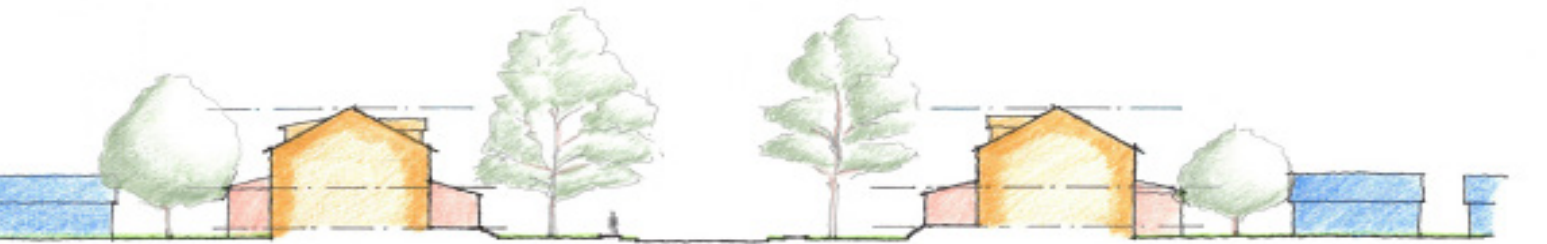
Figure 3. Drexel Avenue section. Note the wider street and slightly shallower setbacks.
