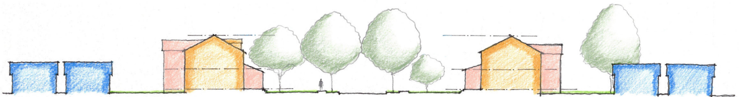
Figure 31. Typical street section. Note the porches, shallow setbacks, and overall compact arrangement.
