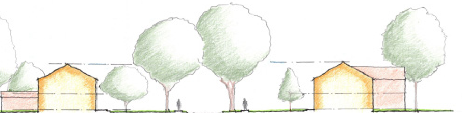
Figure 22. Ashbourne Place section. Note the shallower setbacks compared to the rest of the neighborhood.
