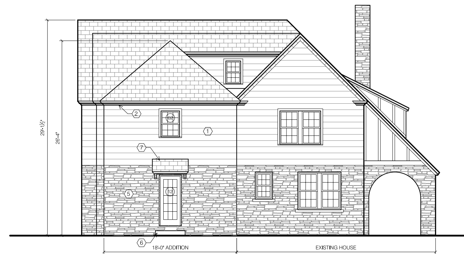
3 NORTH ELEVATION w/ ADDITION SCALE: 1/8" = 1'-0"
