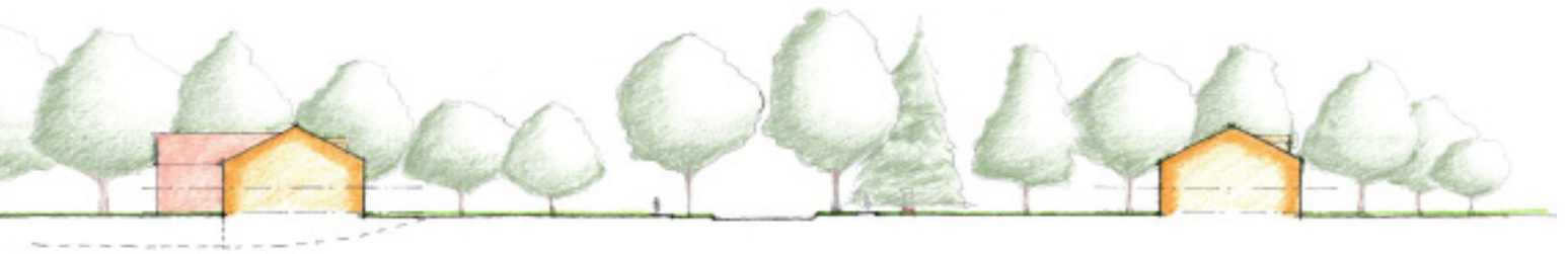
Figure 1. Typical street section. Note the deep setbacks, mature street trees, and abundance of yard trees (front, back, and side). The dashed line on the house to the left shows a condition in which the grade slopes down to a basement-level garage.
