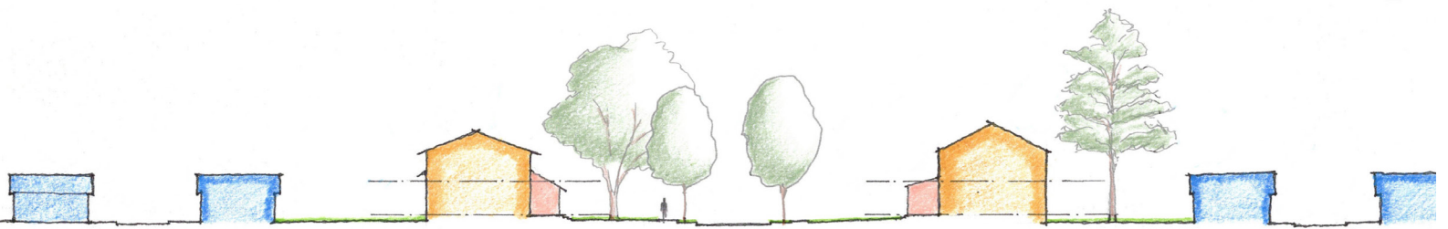
Figure 16. Street section. Note the relatively shallow setbacks, which appear even shallower because of the front porches.
