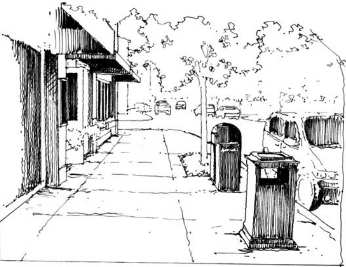
Figure A.3 • Typical Pedestrian Zone - consisting of private amenity zone, minimum 7-foot sidewalk, 6-foot amenity zone and 2-foot curb walk
