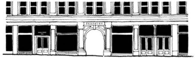
Figure 17.1 • Multiple Storefront Facade - storefront facade shall be divided into narrow bays with entryways recessed into the façade line
