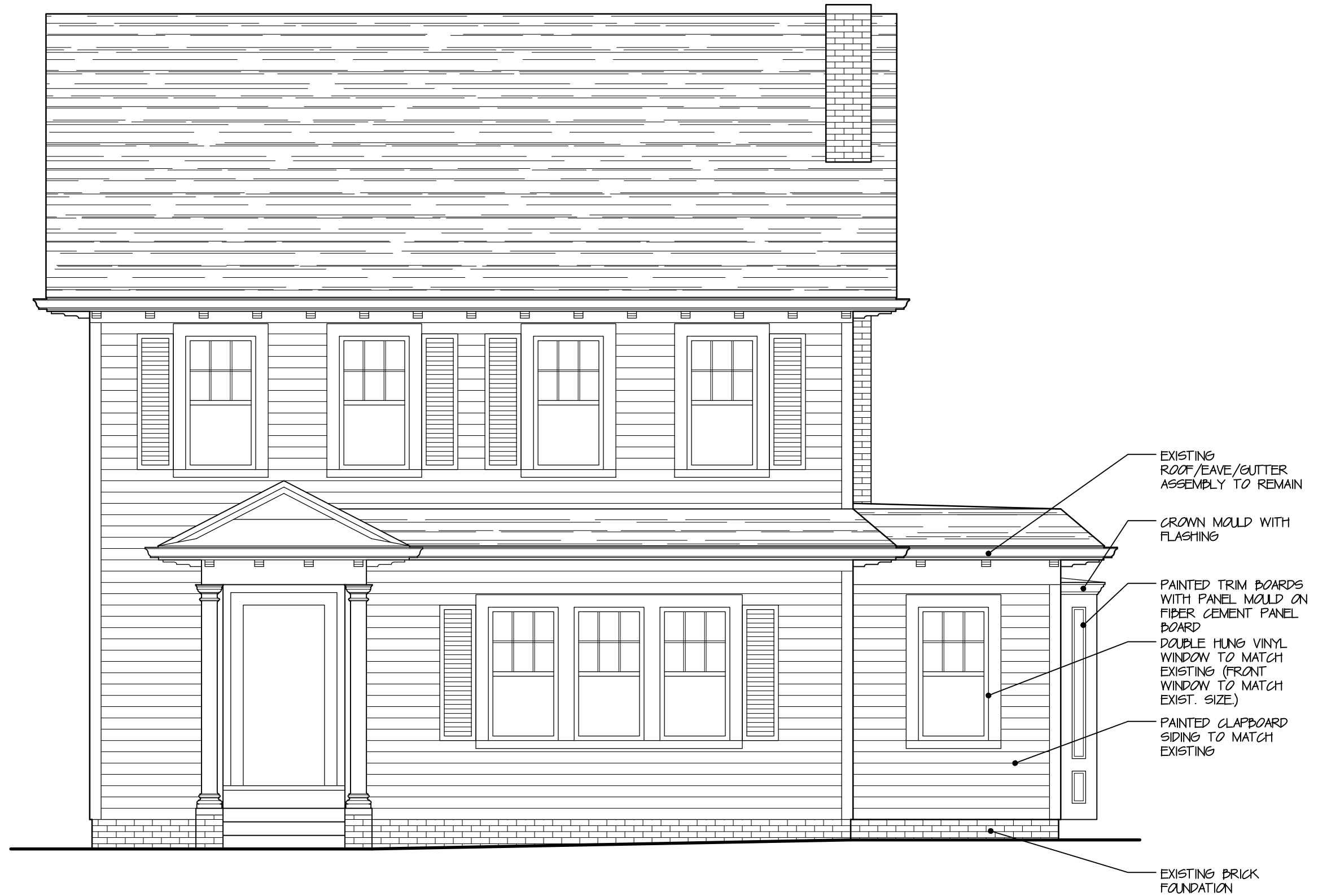
WEST ELEVATION SCALE - 1/4"=1'-0"
