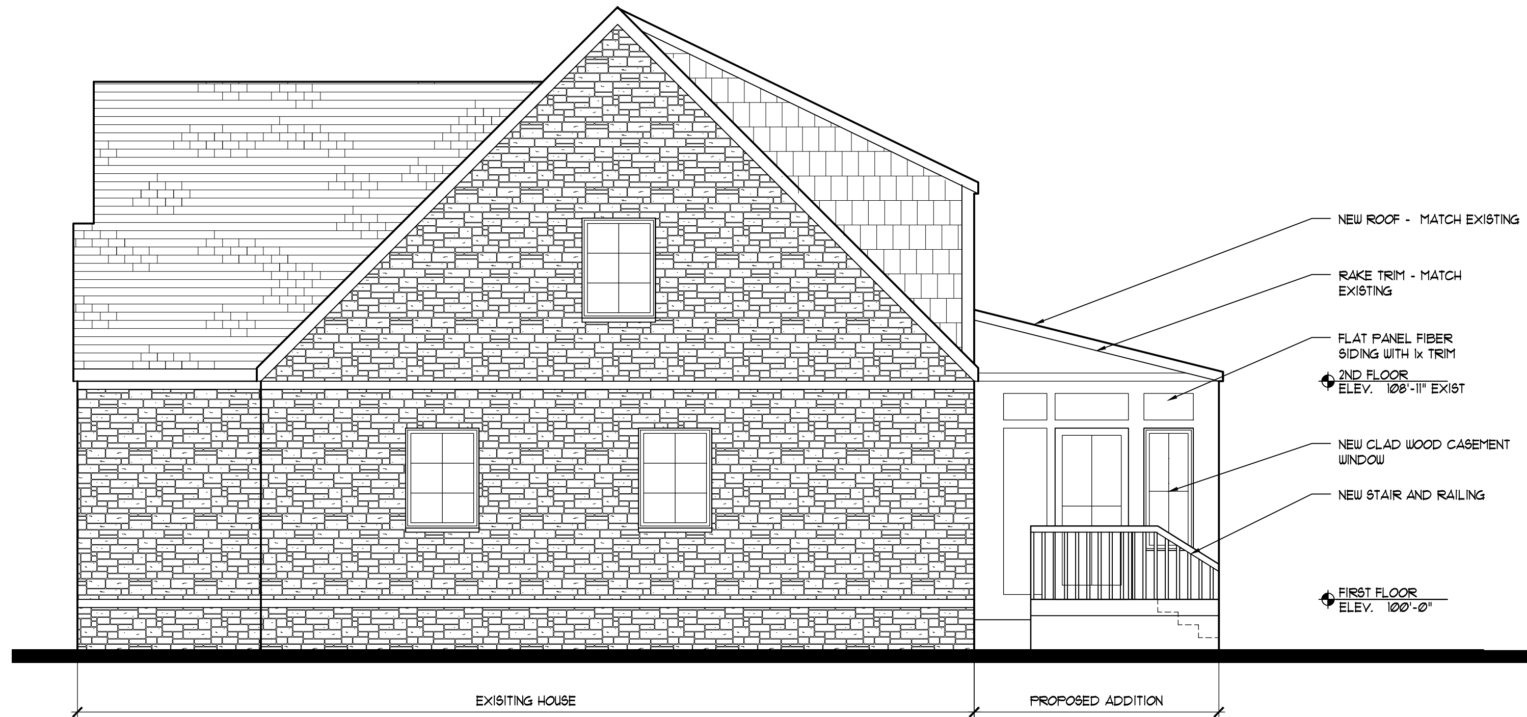
1 SIDE ELEVATION A6 1/4" = 1'-0"
