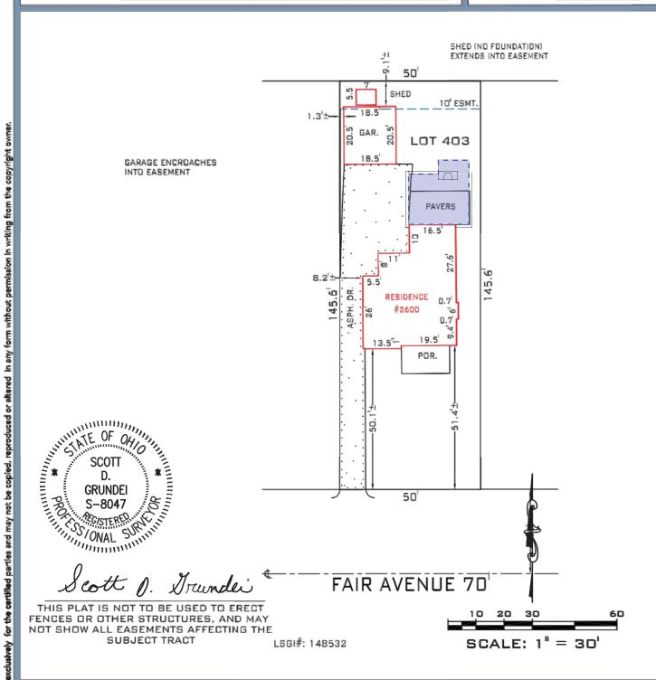
POINTS OF INTEREST: GARAGE ENCROACHES INTO EASEMENT ALSO SHED (NOFOUNDATION) EXTENDS INTO EASEMENT.
