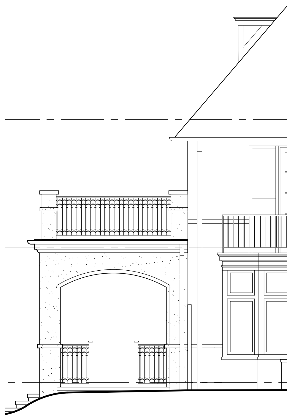
New Covered Front Porch
