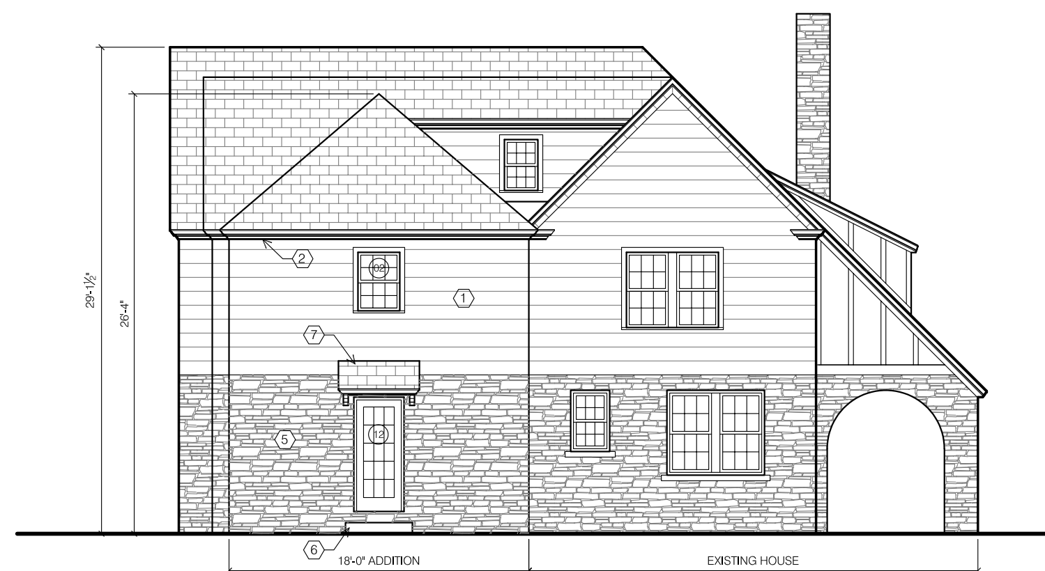
3 NORTH ELEVATION w/ ADDITION SCALE: 1/8" = 1'-0"
