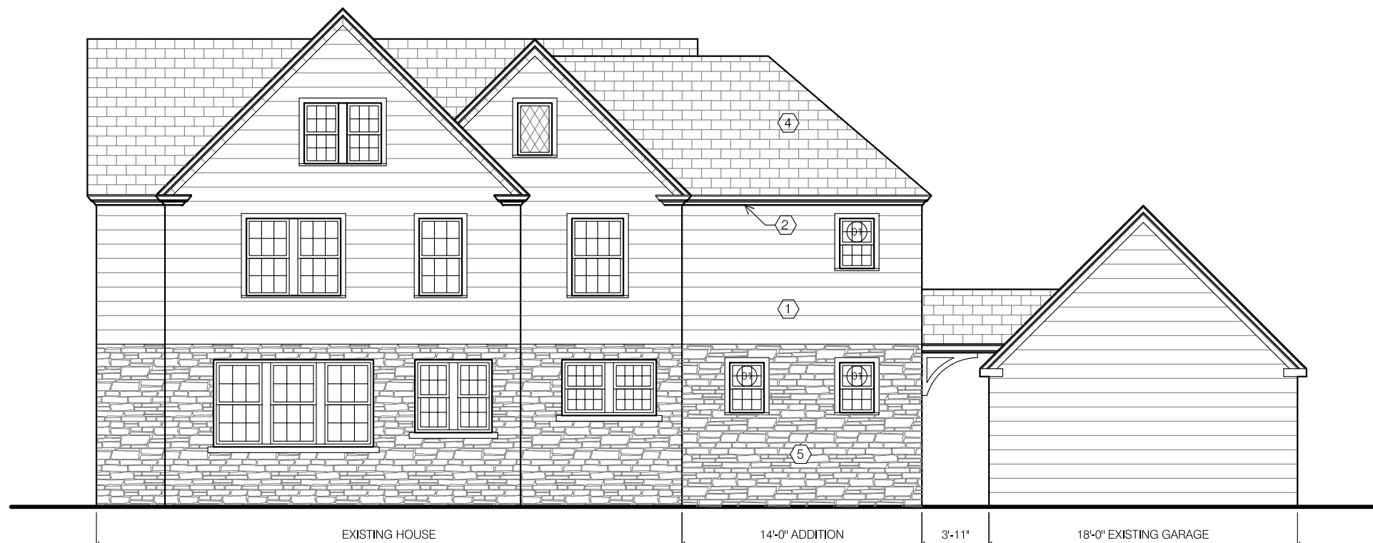
2 EAST ELEVATION w/ ADDITION SCALE: 1/8" = 1'-0"
