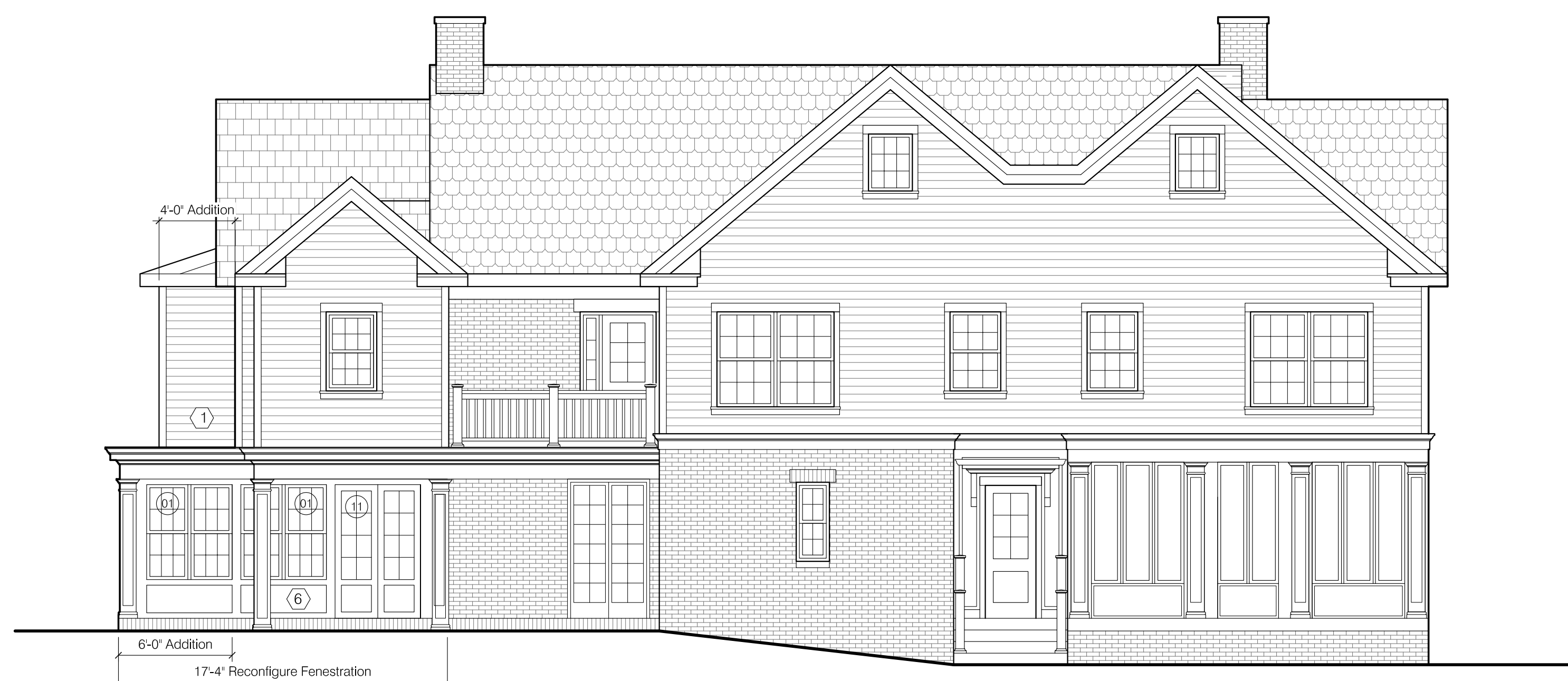
A6 EAST ELEVATION - NEW WORK SCALE: 3/16" = 1'-0"
