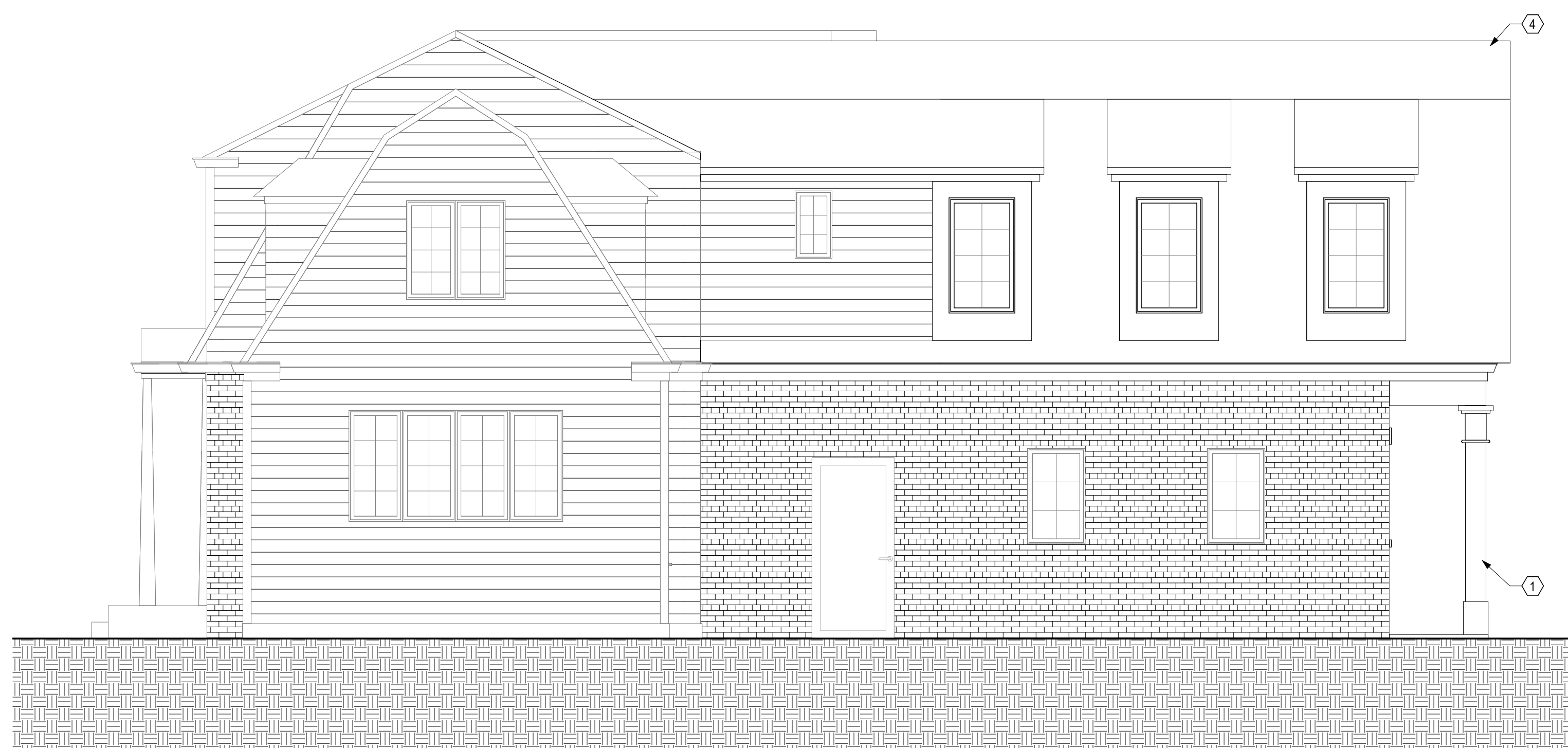
4 ELEVATION WEST - NEW CONSTRUCTION 1/4" = 1'-0" REF: 1 / A201
