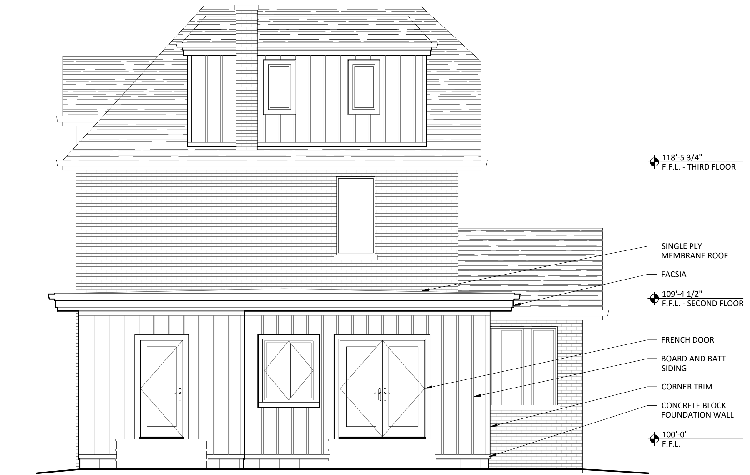
1 A2.2 EXTERIOR ELEVATION - WEST 1/4" = 1'-0"
