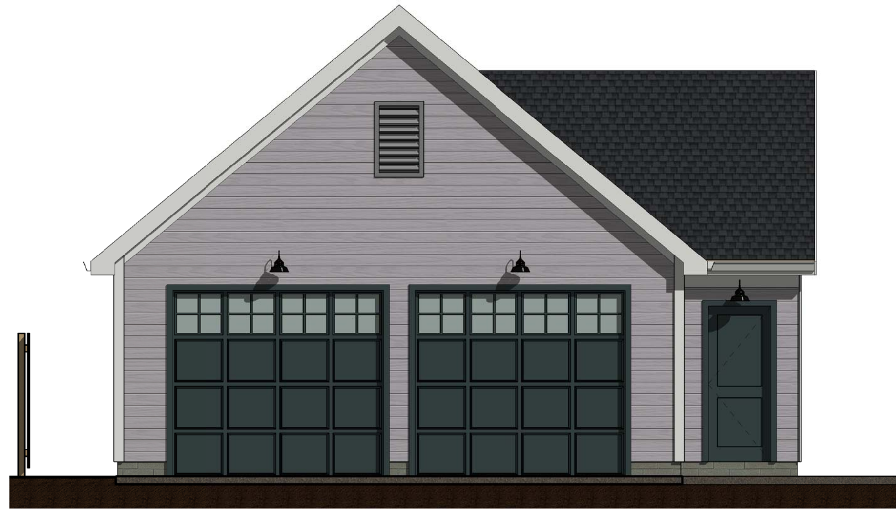
② Garage Front Elevation 1/4" = 1'-0"
