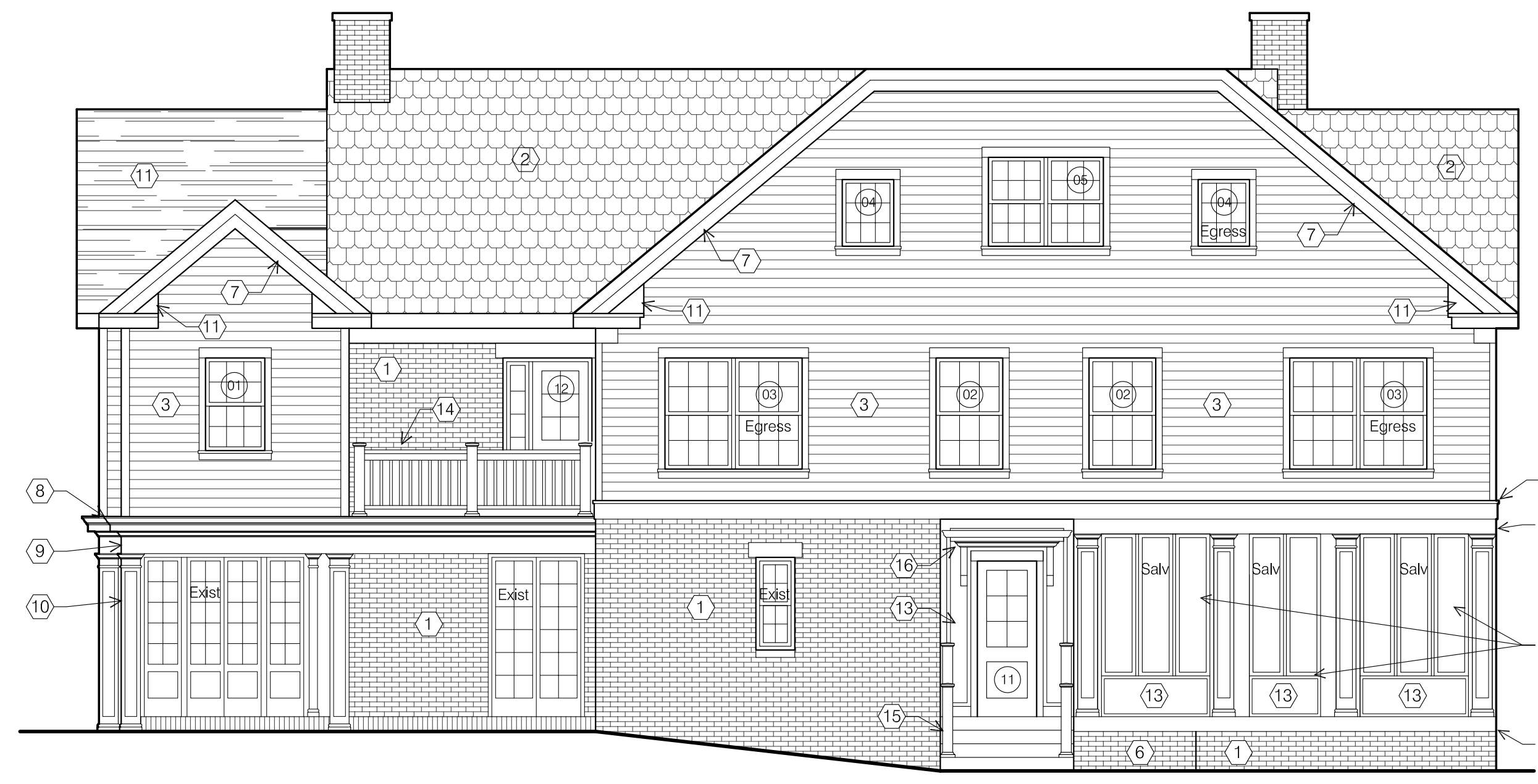
A6 EAST ELEVATION - NEW WORK SCALE: 3/16" = 1'-0" 0 1 2 3 4 5
