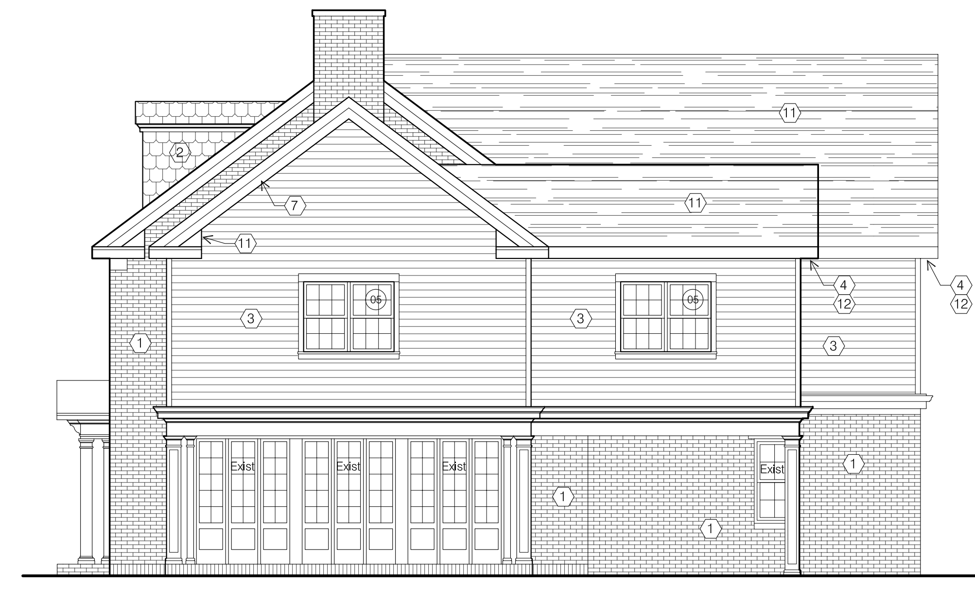
A13 SOUTH ELEVATION - NEW WORK SCALE: 3/16" = 1'-0" 0 1 2 3 4 5
