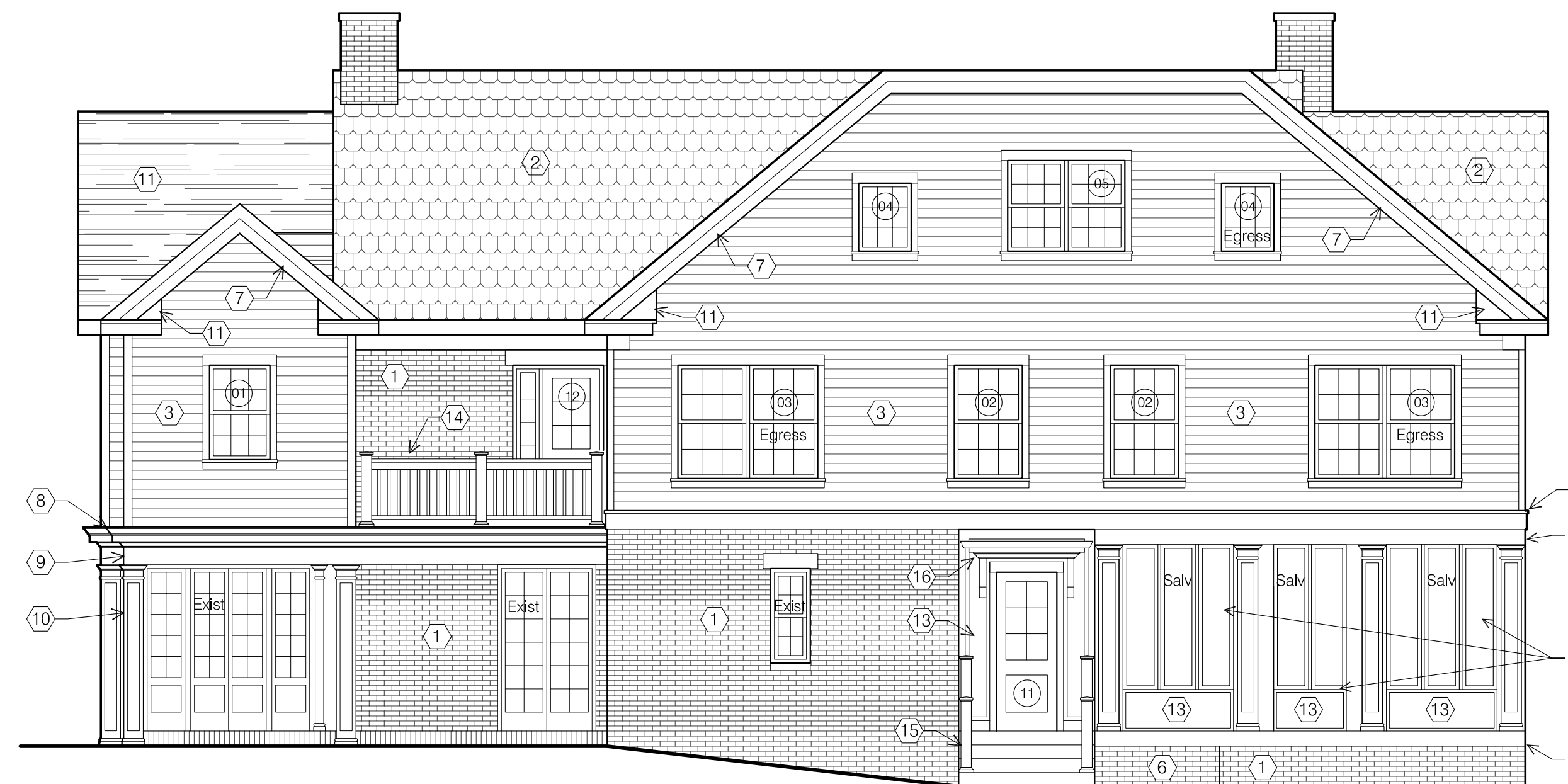
A6 EAST ELEVATION - NEW WORK SCALE: 3/16" = 1'-0" 0 1 2 3 4 5
