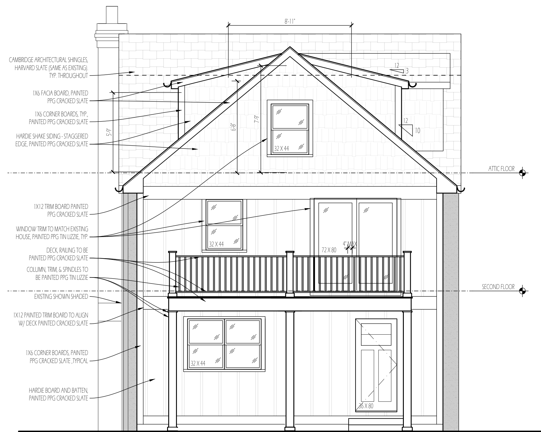
REAR EXTERIOR ELEVATION OF ADDITION
