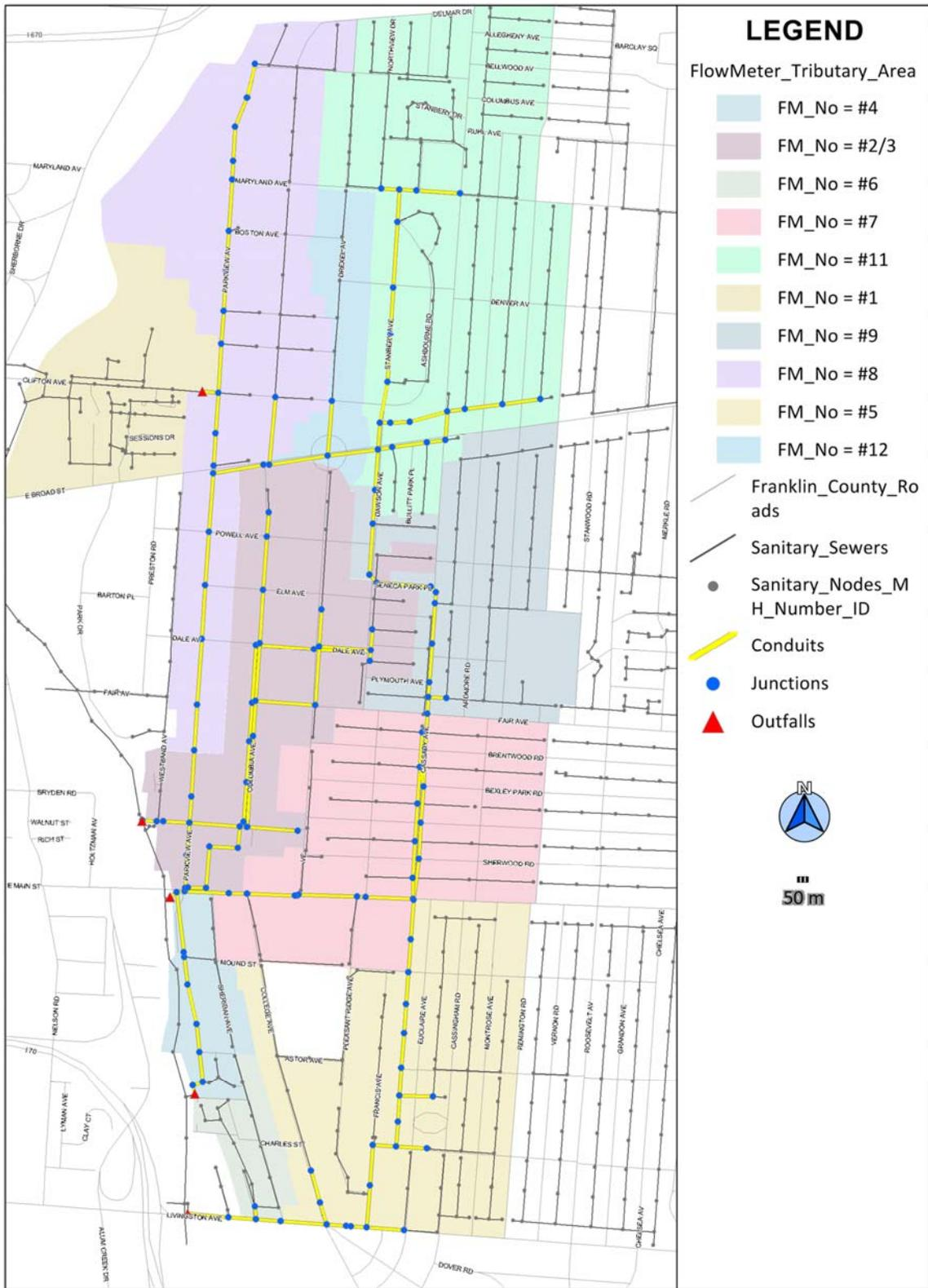
Figure 5-1: Modeled System for City of Bexley
