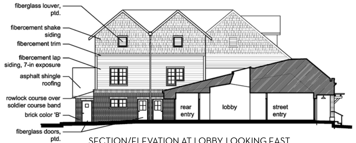
SECTION/ELEVATION AT LOBBY, LOOKING EAST
