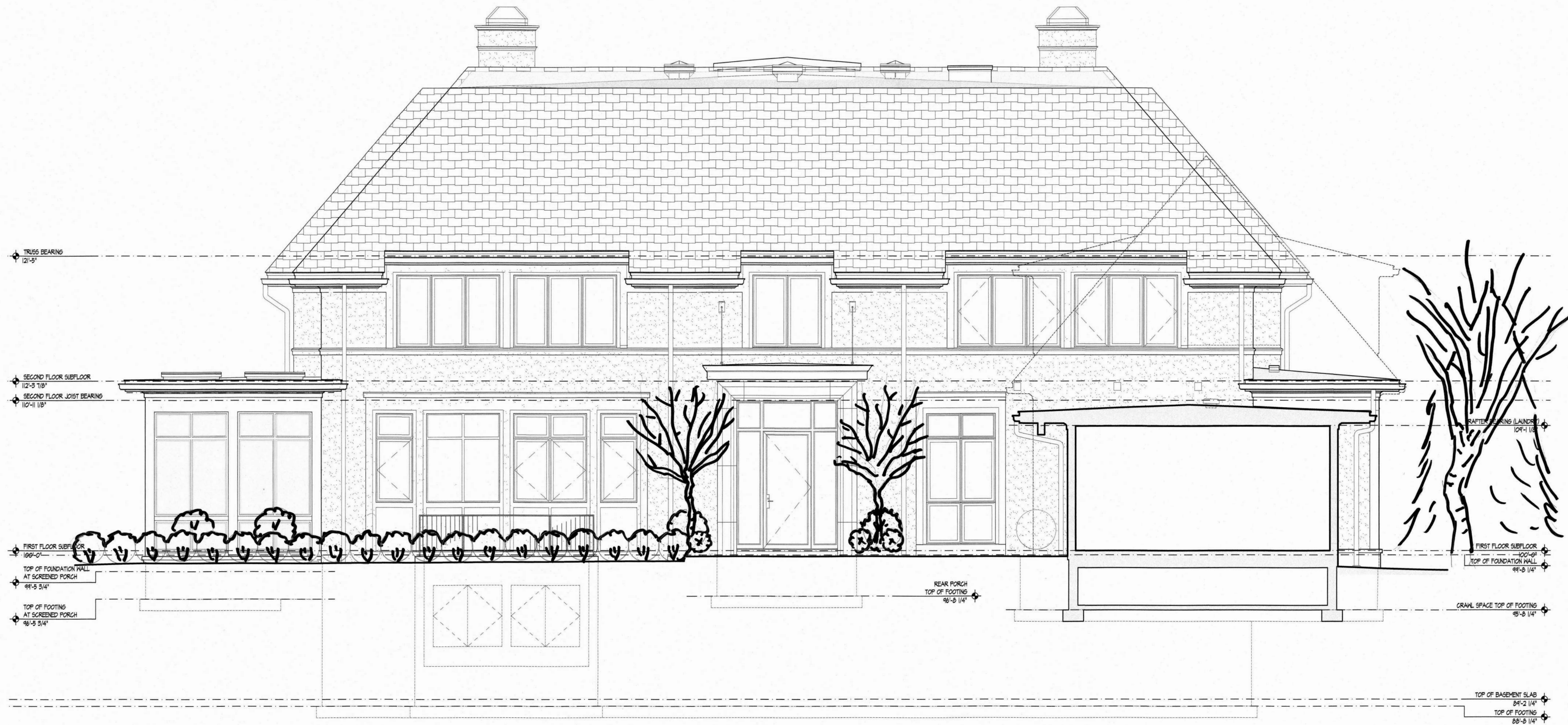
EXTERIOR ELEVATION (EAST VIEW WITH ATTACHED GARAGE SHOWN DASHED) D5 SCALE: 1/4" = 1'-0"
