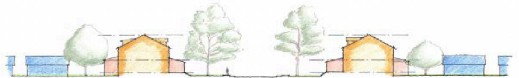
Figure 3. Drexel Avenue section. Note the wider street and slightly shallower setbacks.
