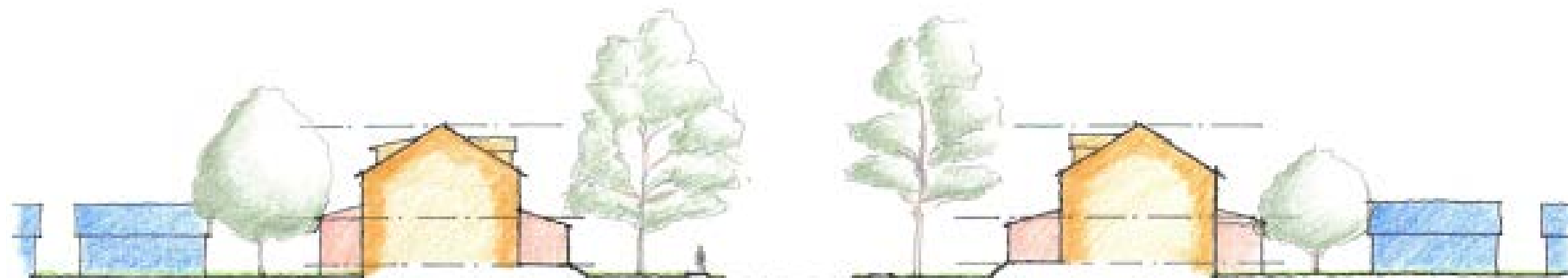
Figure 4. Bullitt Park Place section. Note the compact arrangement of the lot and the shallow setbacks.
