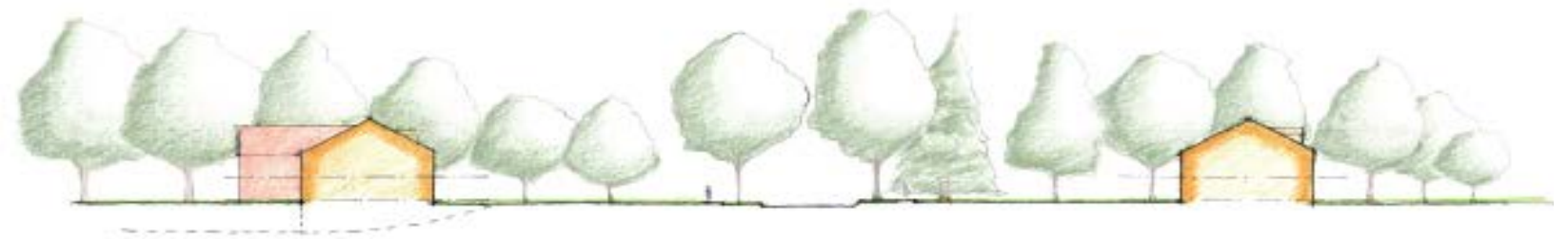
Figure 1. Typical street section. Note the deep setbacks, mature street trees, and abundance of yard trees (front, back, and side). The dashed line on the house to the left shows a condition in which the grade slopes down to a basement-level garage.
