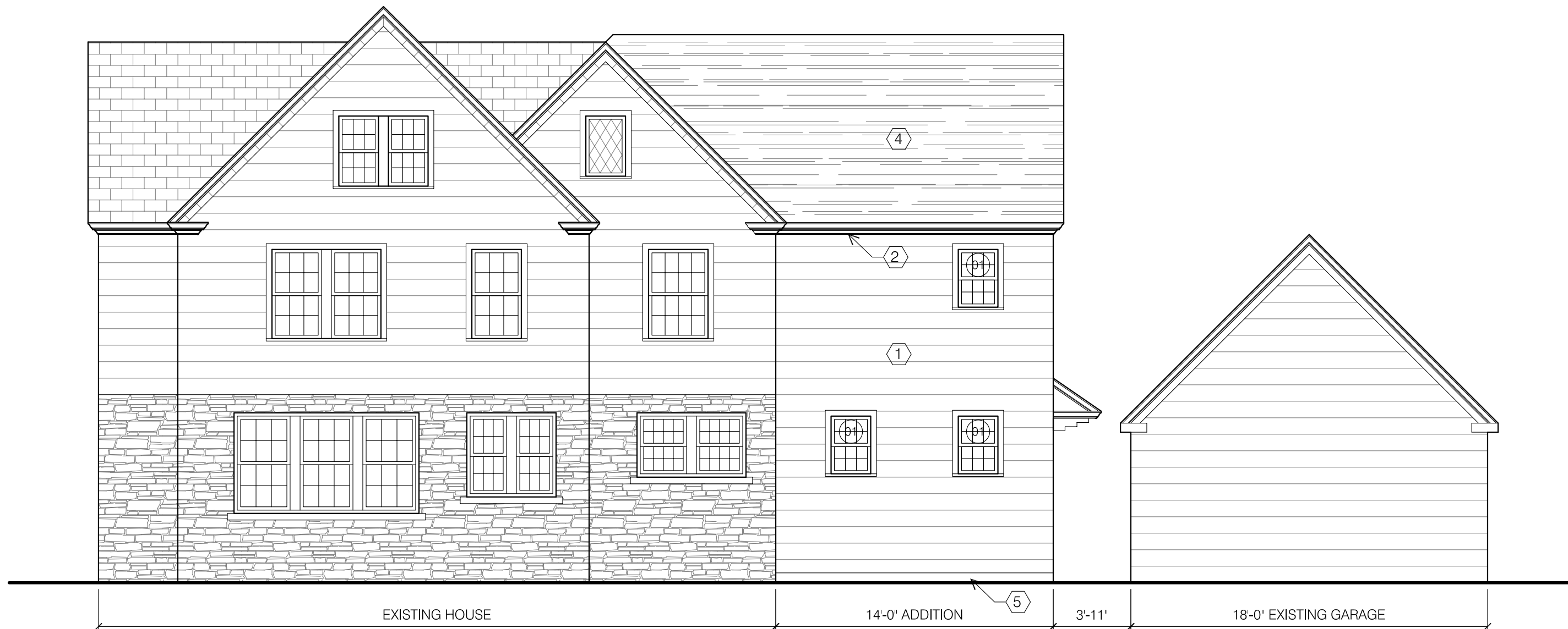
A2 EAST ELEVATION w/ ADDITION SCALE: 3/16" = 1'-0" 0 1 2 4 8
