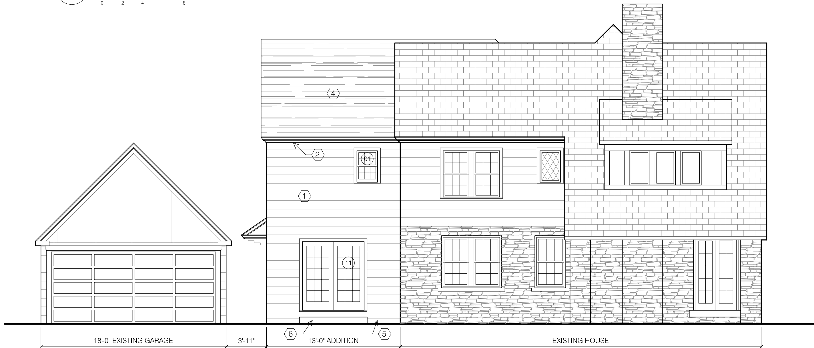
A2 WEST ELEVATION w/ ADDITION SCALE: 3/16" = 1'-0" 0 1 2 4 8
