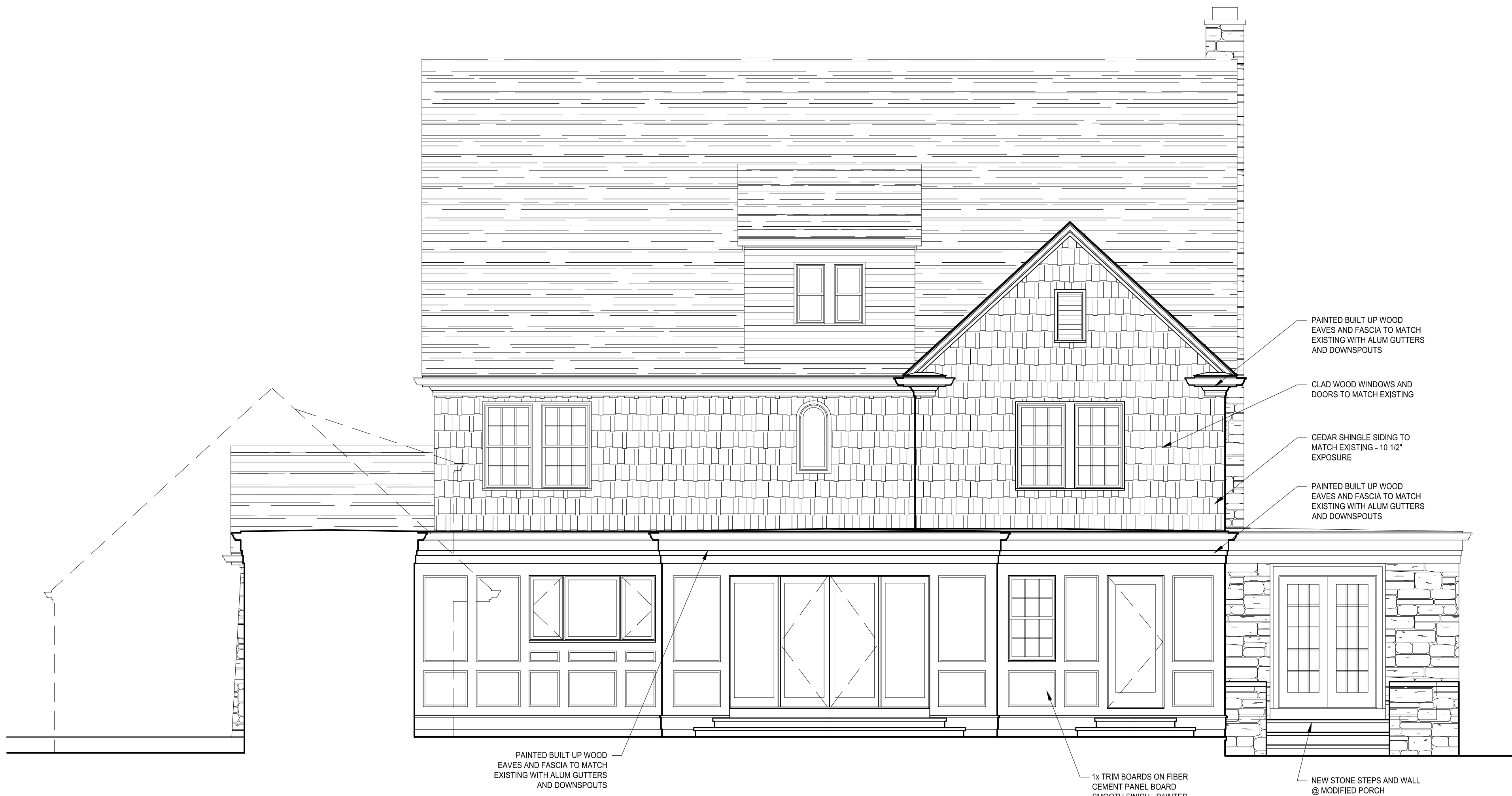
PROPOSED WEST ELEVATION 1/4" = 1' - 0"
