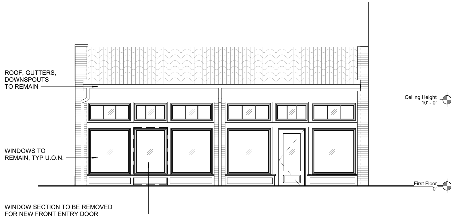
1 NORTH ELEVATION - EXISTING SCALE: 3/16" = 1'-0"
