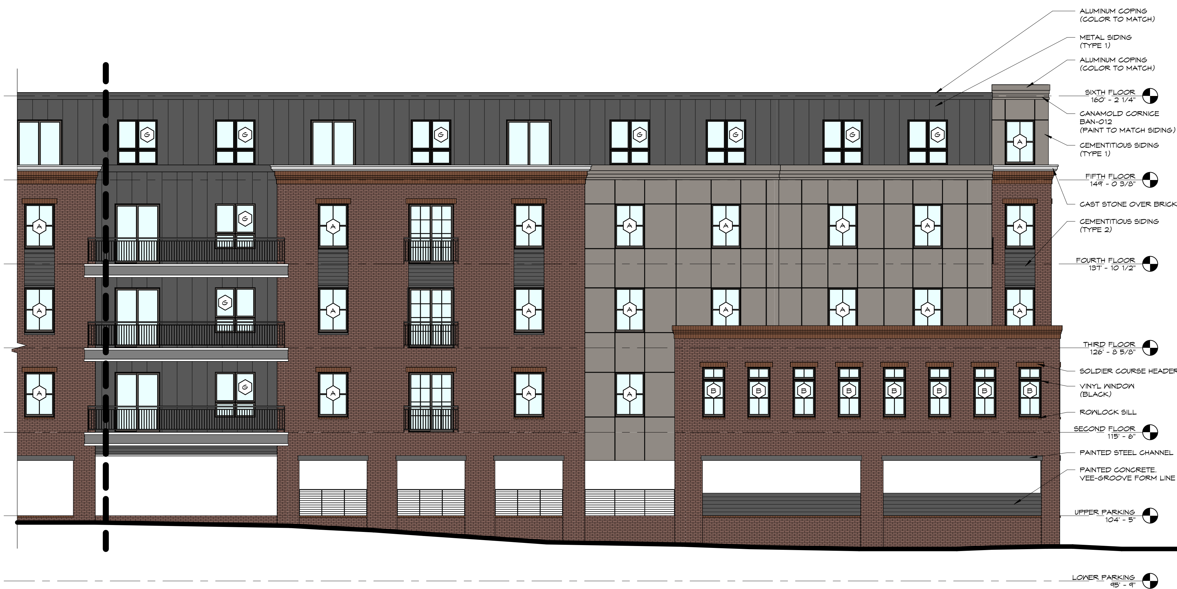
F3 PARTIAL NORTH ELEVATION 1/8" = 1'-0"
