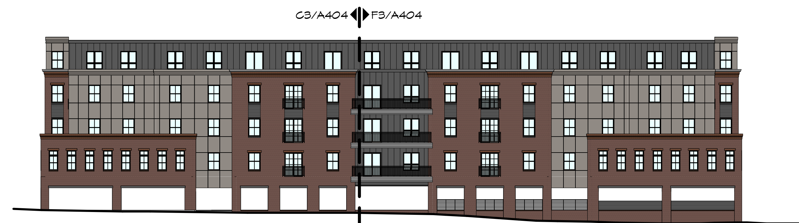
G3 OVERALL NORTH ELEVATION 1" = 20'-0"
