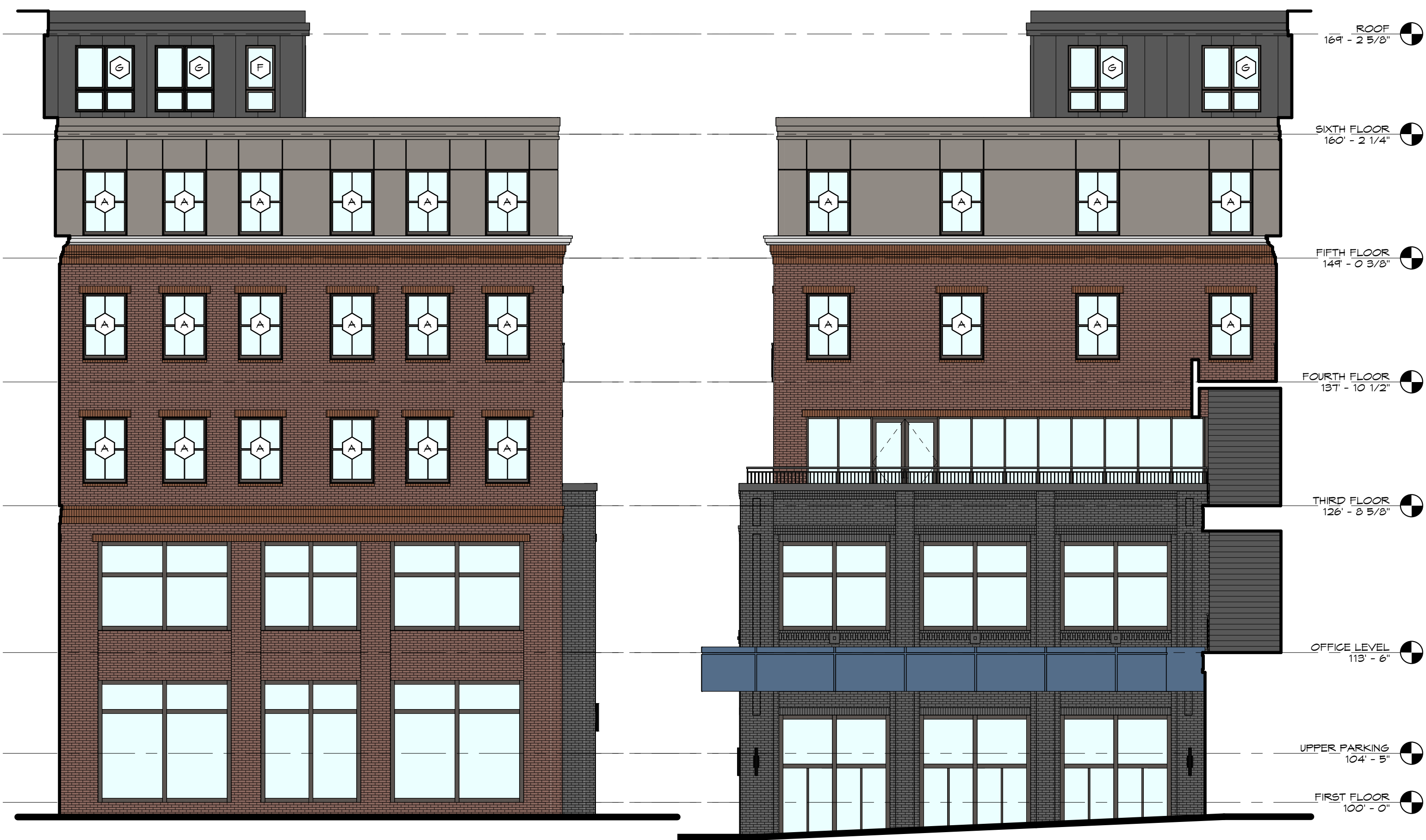
F8 WEST COURTYARD ELEVATION 1/8" = 1'-0"
