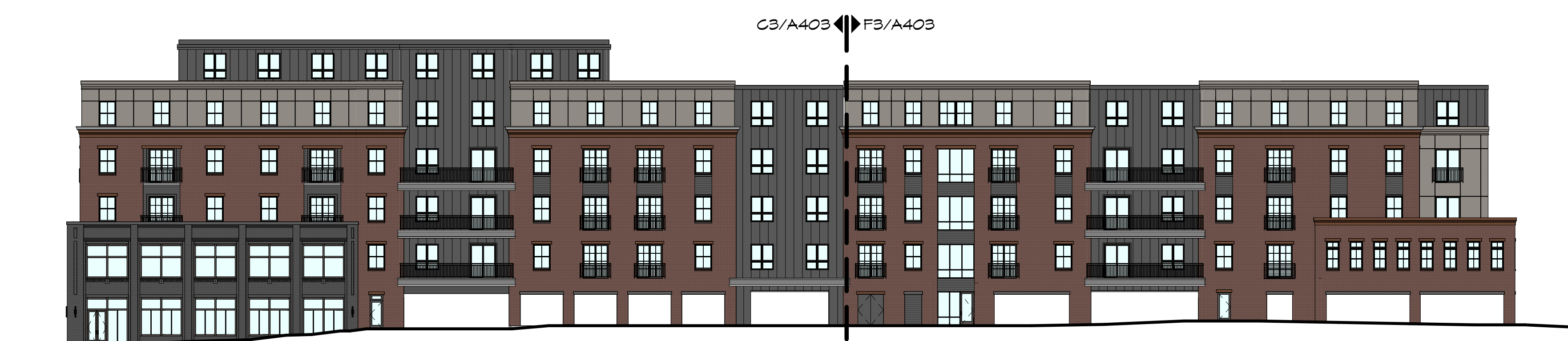
G3 OVERALL EAST ELEVATION 1" = 20'-0"
