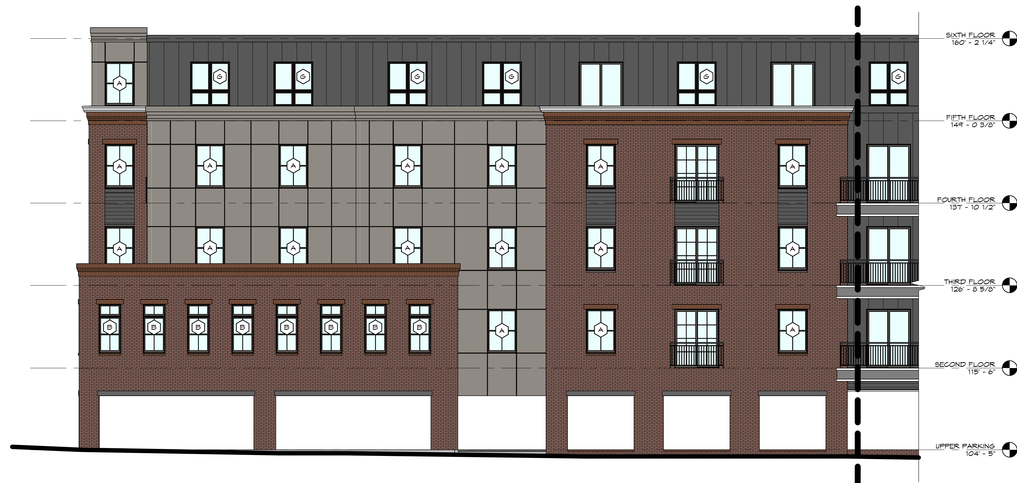
C3 PARTIAL NORTH ELEVATION 1/8" = 1'-0"
