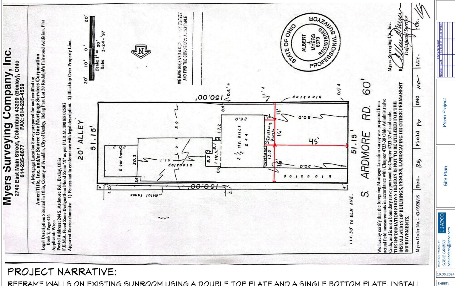
REFRAME WALLS ON EXISTING SUNROOM USING A DOUBLE TOP PLATE AND A SINGLE BOTTOM PLATE. INSTALL NEW MARYIN GLIDER AND PICTURE WINDOWS
