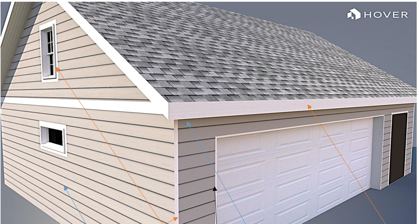
7" reveal siding 5/4" x 4" corners, window/ door trims and frieze (frieze not shown) 4/4" x 8" fascia
