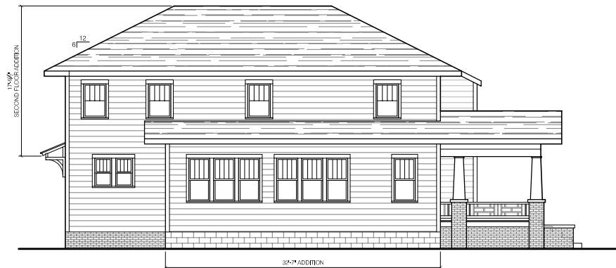
SOUTH ELEVATION - w/ ADDITION Front Bay Roof tucks under main hip roof
