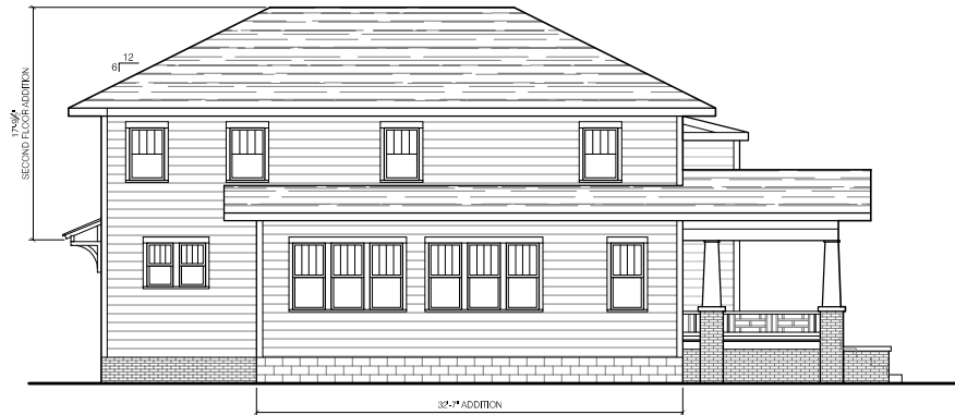
SOUTH ELEVATION - w/ ADDITION Hip roof extends to pick up front bay
