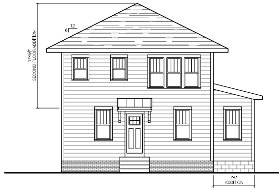
WEST ELEVATION - w/ ADDITION Gable end at single-story addition
