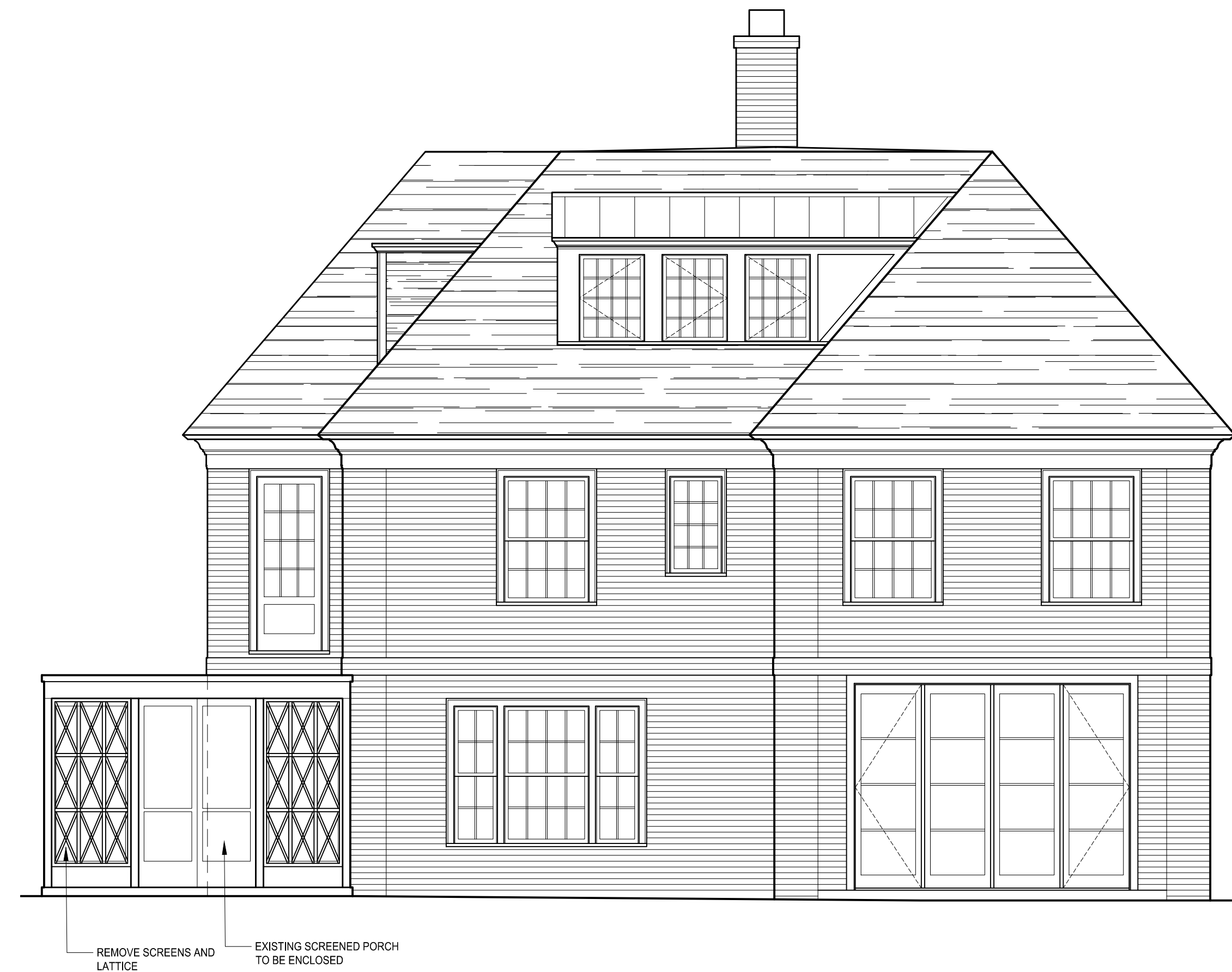
A A2.1 EXISTING SOUTH ELEVATION 1/4" = 1'-0"
