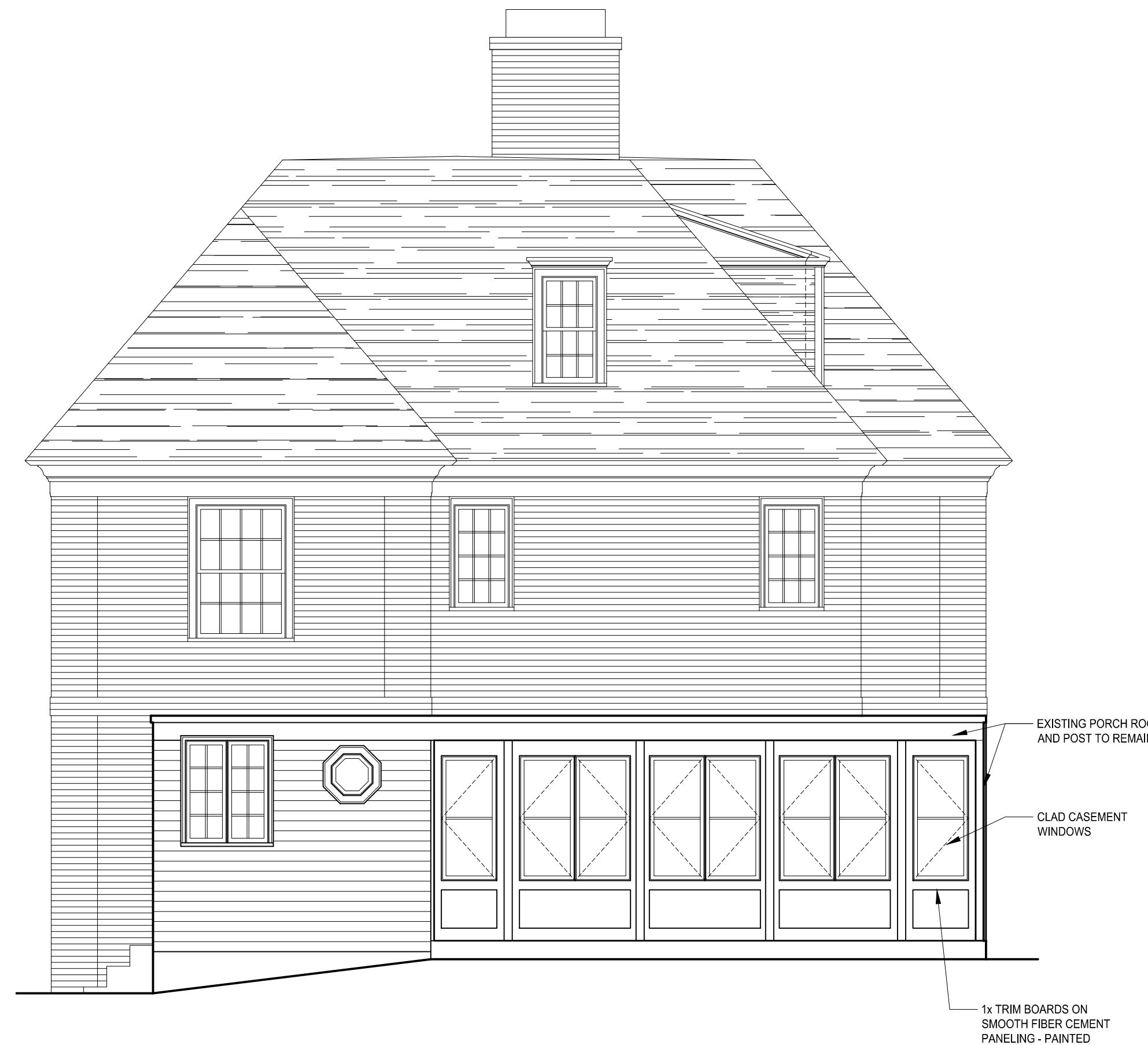
D A2.1 PROPOSED WEST ELEVATION 1/4" = 1'-0"
