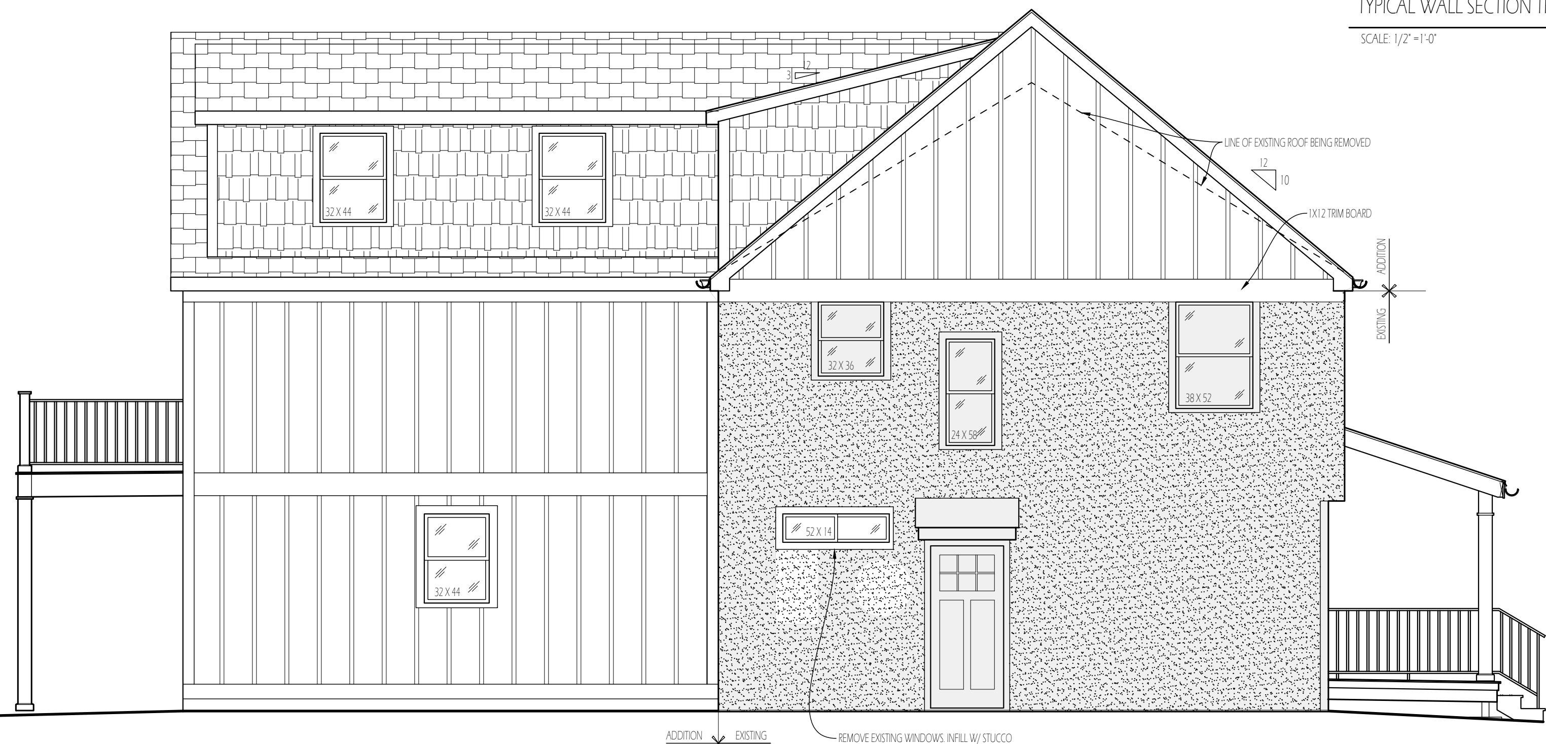
REAR EXTERIOR ELEVATION OF DETACHED GARAGE SCALE: 1/4" = 1'-0"
