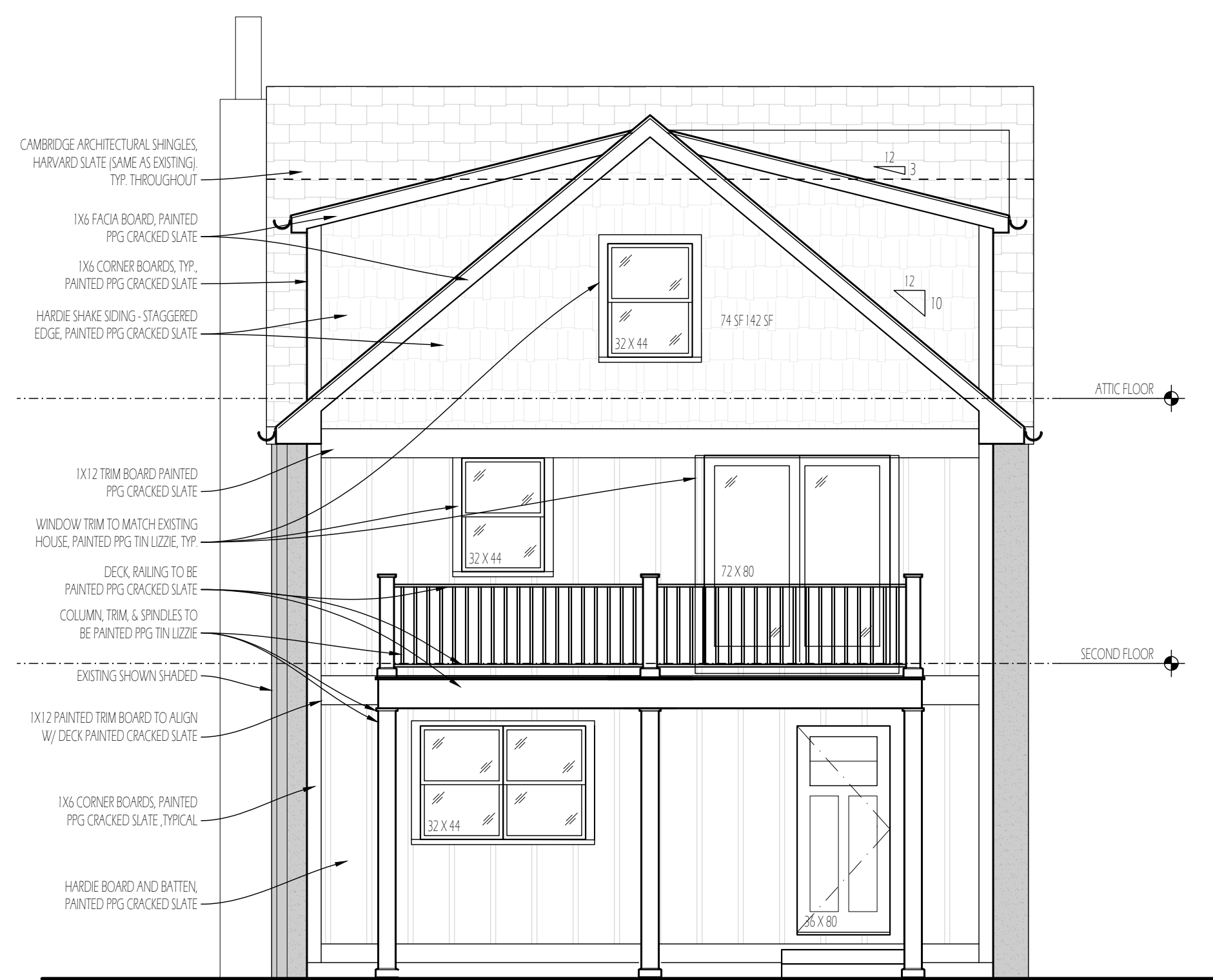
REAR EXTERIOR ELEVATION OF ADDITION SCALE: 1/4" = 1'-0"
