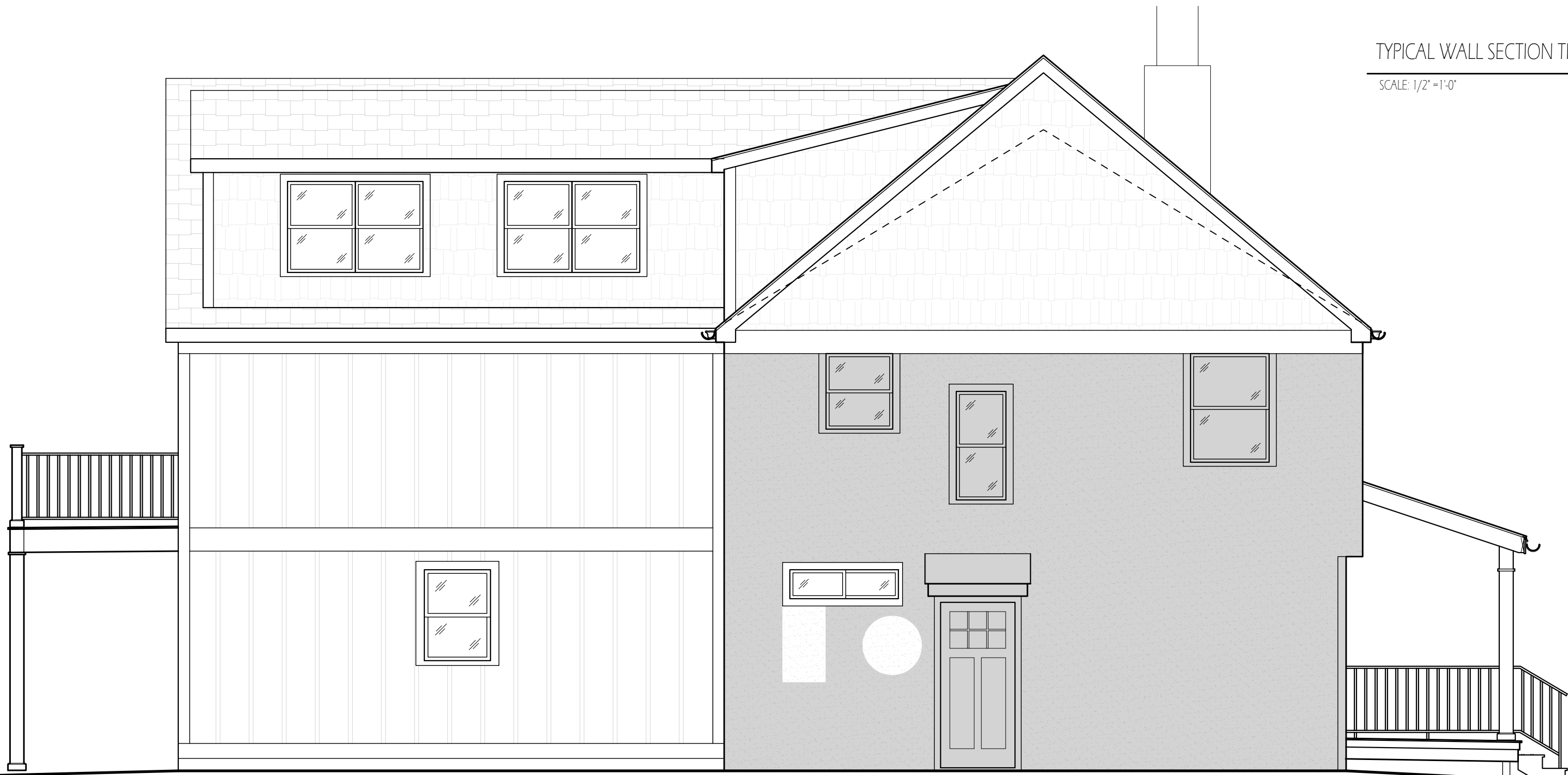
REAR EXTERIOR ELEVATION OF DETACHED GARAGE SCALE: 1/4"=1'-0"
