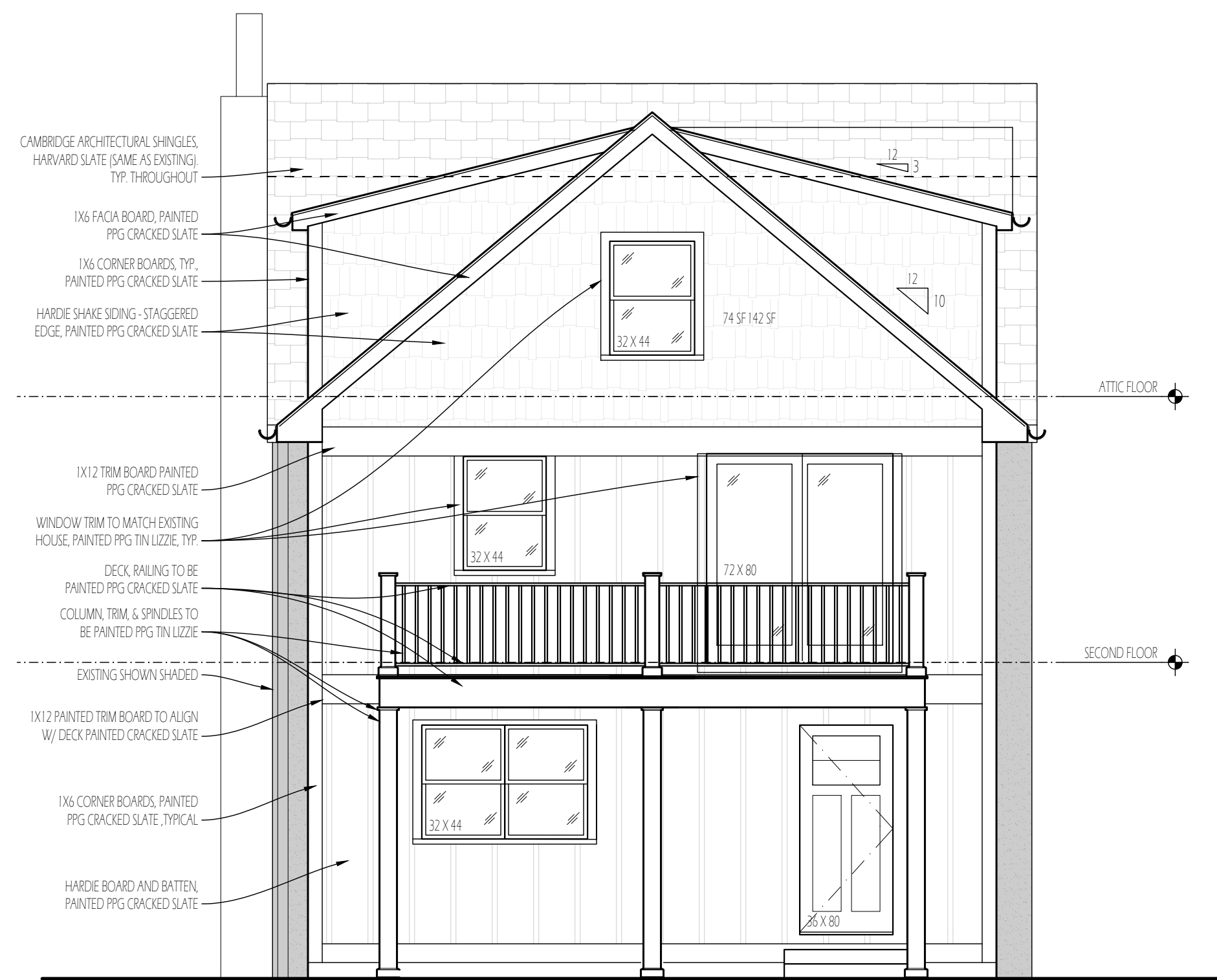
REAR EXTERIOR ELEVATION OF ADDITION SCALE: 1/4" = 1'-0"
