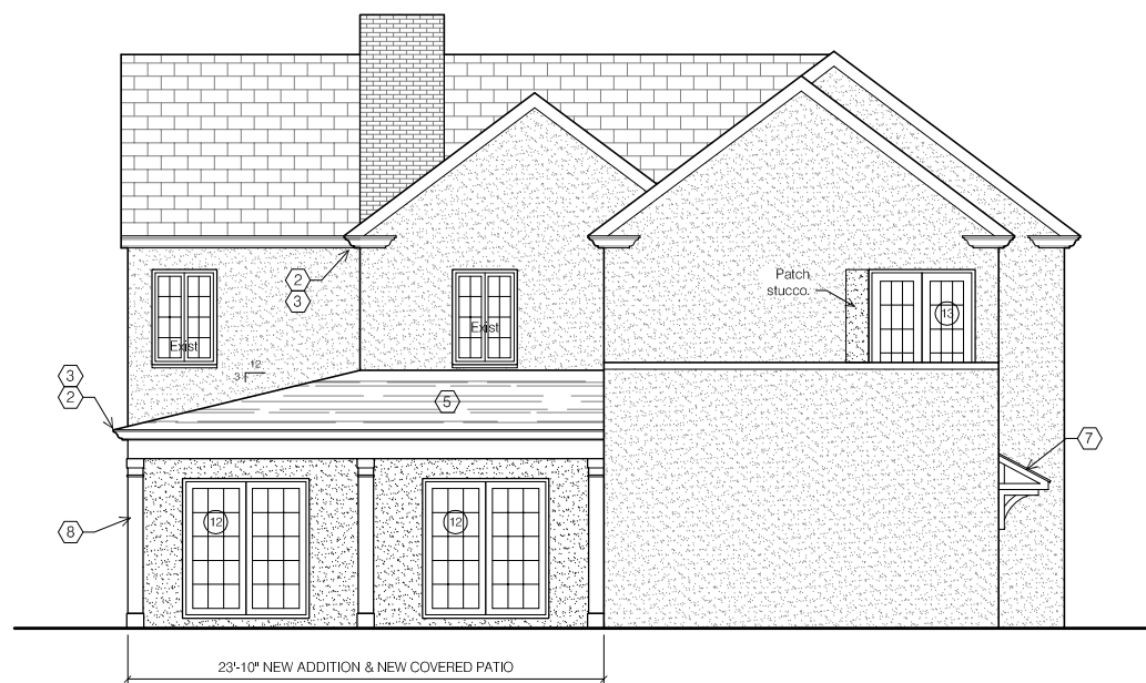
SOUTH ELEVATION - NEW WORK
