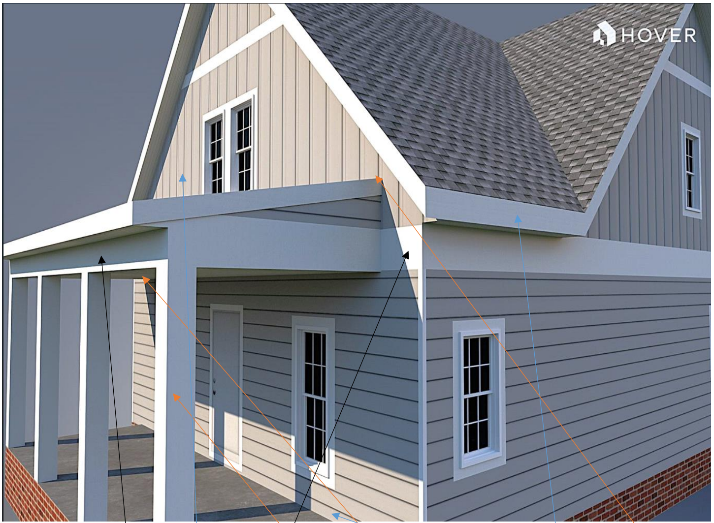
12" O.C. board and batten siding porch columns and ceiling by others 4/4" x 8" fascia 5/4" x 10 header wraps and lower band boards 5/4" x 6" Boral used against concrete and 4" against roofline
