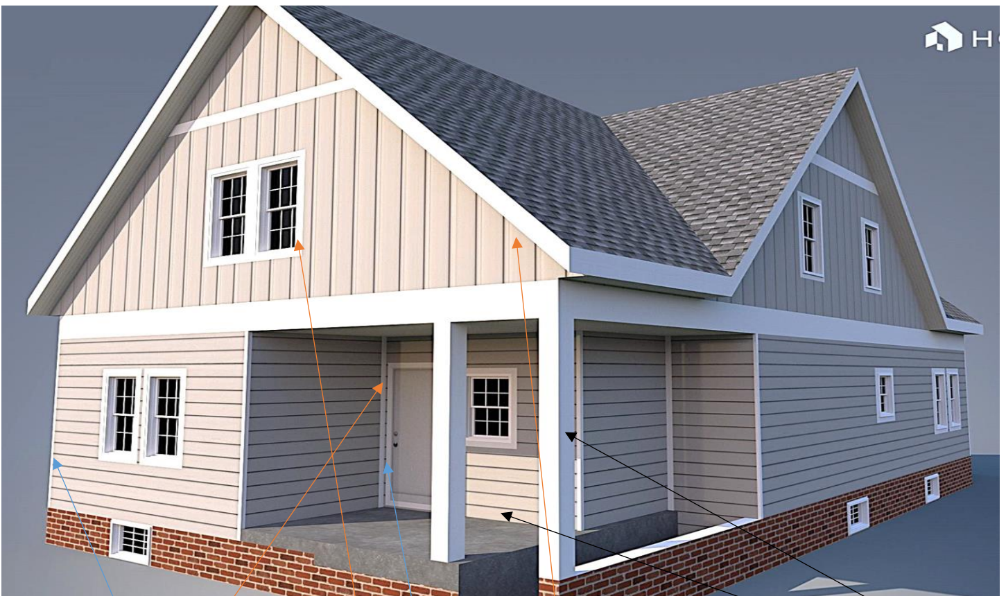
5/4" x 4" outside/ inside corners, window/ door trims and frieze 5/4" x 6" Boral against concrete columns by others
