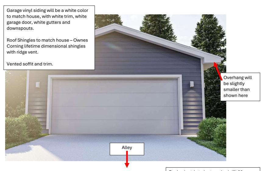
Basic electric to be trenched, (2) 20amp circuits from new home meter socket to new garage. 2 interior outlets, 2 interior lights, 2 exterior lights, and Liftmaster/Chamberlain wifi garage door opener with remotes.
