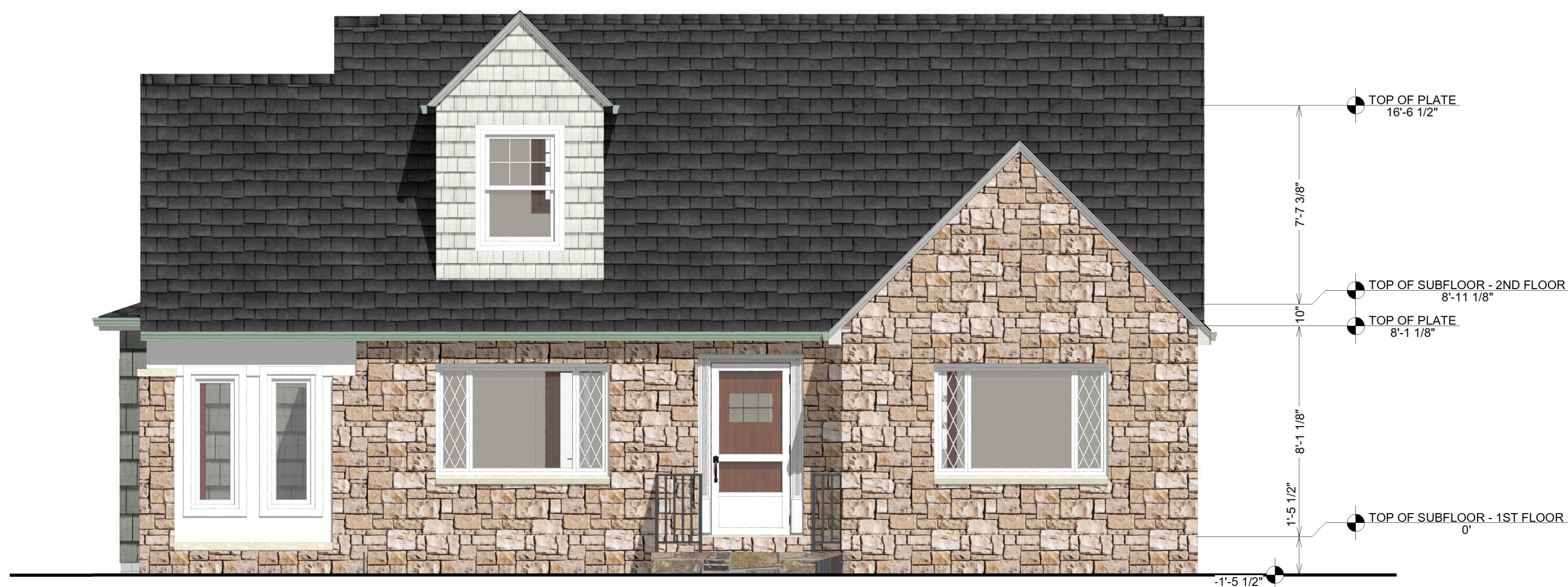
02 EXISTING FRONT ELEVATION 1/4" = 1'-0"
